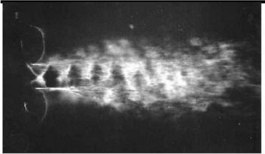
Schlieren Visualization of Shocks and Expansions in a Plane Jet
